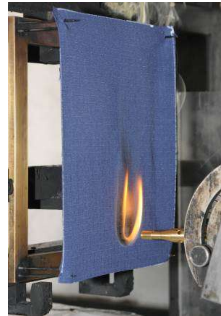
Illustration of edge ignition (ISO 15025)
